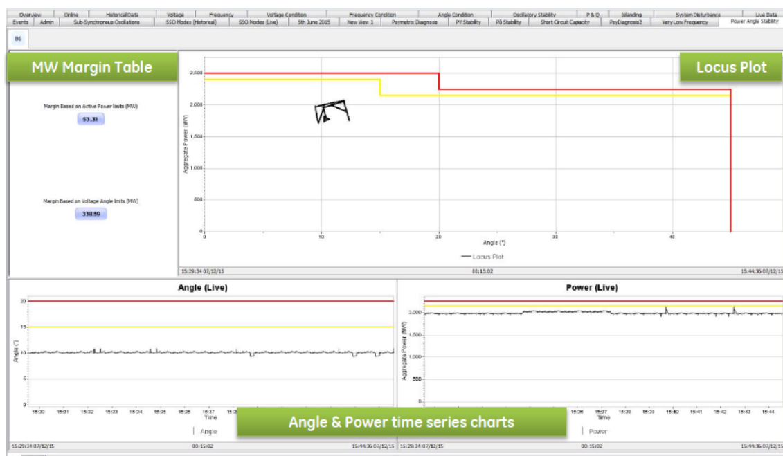
Figure 11. Boundary constraint application in PhasorPoint
